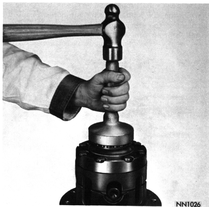
Fig. 9—Installing Differential Bearing Cones
